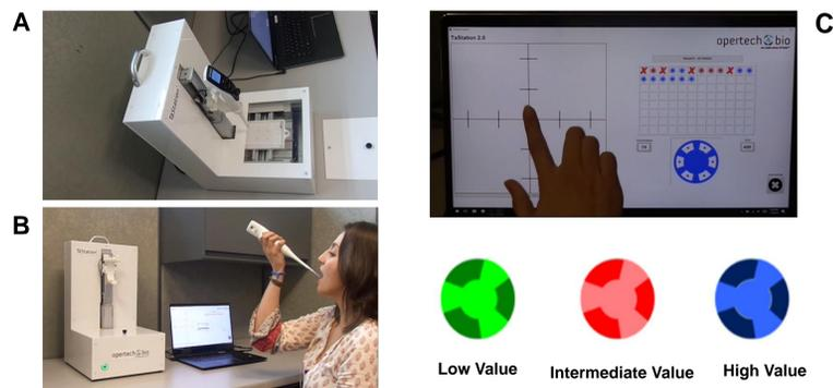
A) Robotic pipette randomly selects a well from a 96-well plate, withdraws 0.2 ml and presents pipette to subject
