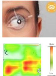
Participants in the study were fitted with a Galvanic Skin Response (GSR) Shimmer kit that produces peak signals based on skin conductance during sweating. Two cameras collected facial recognition data. The Affective module within the iMotions software package was used to identify facial action units or individual expressions to classify emotional states. Eye tracking data was also collected
